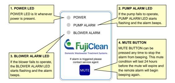
Normally when the system is operating correctly, only the green POWER LED is lit to indicate that power is available.
