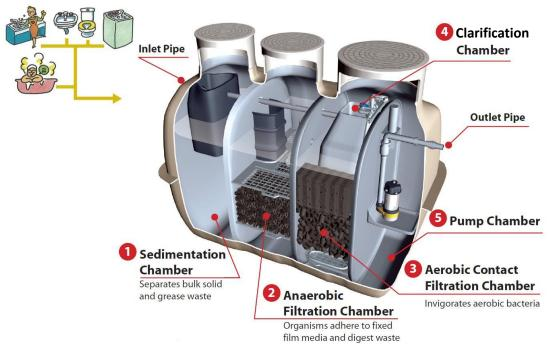
CE-1500EX is designed to treat all household wastewater from the kitchen, bathroom, toilet and laundry area and is capable of producing Advanced Secondary Quality Effluent as specified below. The daily design flow rate of CE-1500EX is 1,500 L/day.
